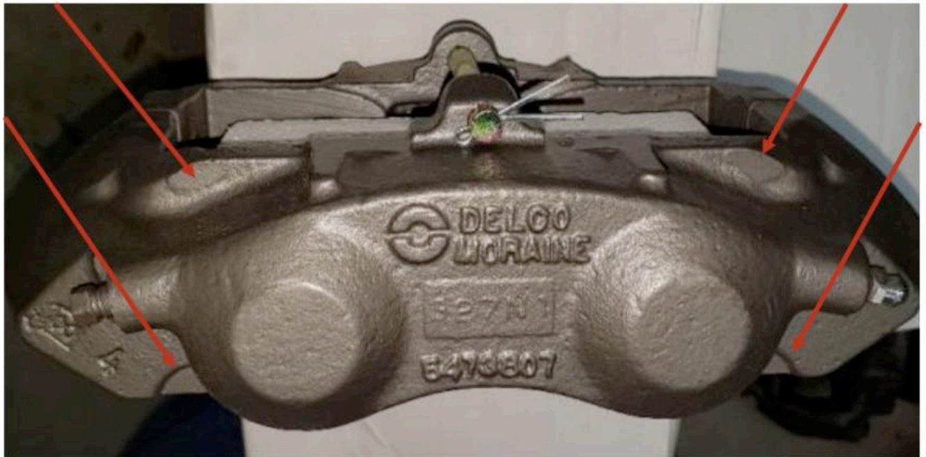
Fig. #1. RF Caliper side. Red arrows show semi-circles that were spot faced, leaving no paint.
